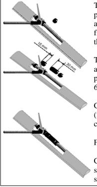
This System allows the pilot to vary the speed and precision of the kite by moving a pair of spacers above or below the lower spreader - leading edge fittings. This changes the effective stand off lengths, the kites aspect ratio and the bridles position.
